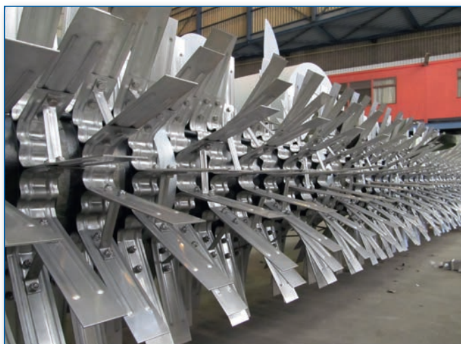
Brush aerator ready for transport
