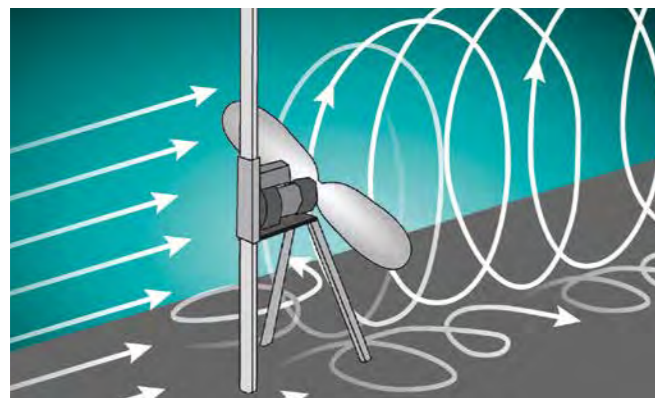
High-loss high-vortex flow induced by conventional horizontal flow generators
